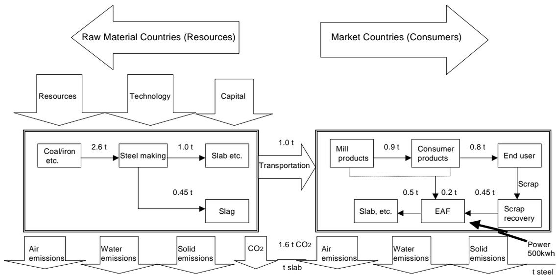
**Figure 5. Steel Making and Products Life Cycle**
