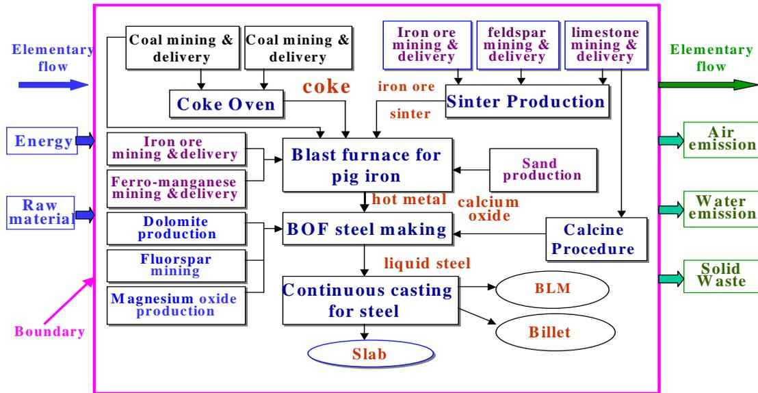
Figure 3. Unit process within Steel LCI System - Integrated Steel Mill[1]
