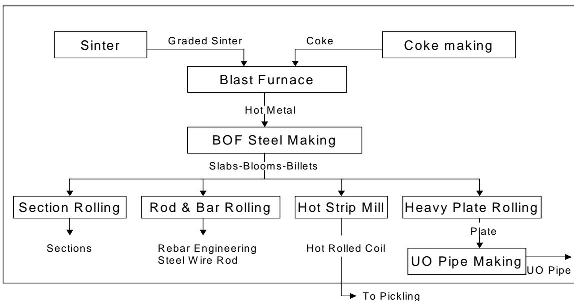
**Figure 2. Steelmaking : Blast Furnace Route**
