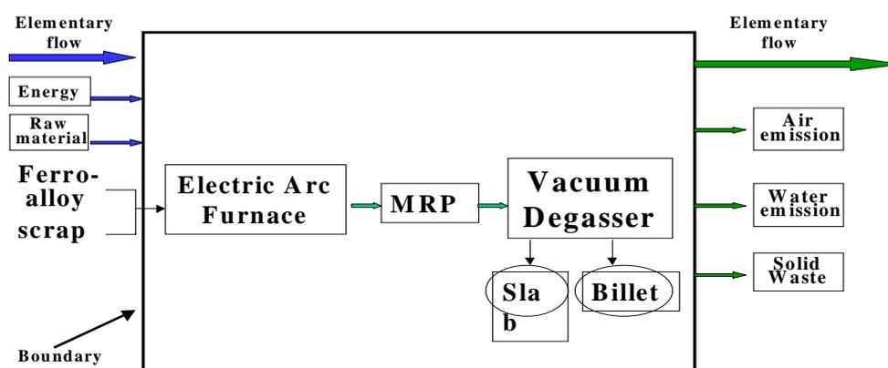
Figure 4. Unit process within Steel LCI System
